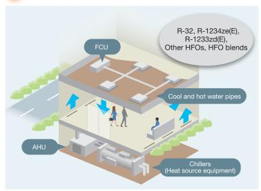
Chilled/hot water generated by a chiller and heat pump passes through the pipes in a building and enters terminal units such as Air Handling Units (AHU) and Fan Coil Units (FCU) to cool/heat air. Chillers are typically located in the mechanical room or on the roof. It is important to select appropriate refrigerants that are suitable for various compressor types and applications depending on system and capacity.
