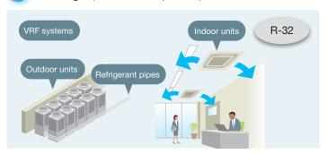
Multi-split packaged air conditioners for commercial buildings that use variable refrigerant flow enable a connection of multiple indoor units to outdoor units and individual climate control settings for each zone. Daikin has identified R-32 as the most appropriate refrigerant for this type of equipment.
