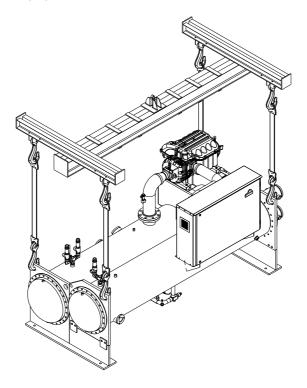
Figure 2 - Lifting the unit
