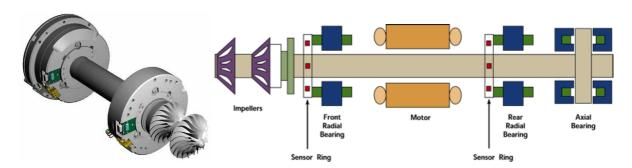
The compressor speed adjusts to changes in load and/or condensing temperature. As compressor speed reduces due to lower loads and /or condensing temperatures, energy consumption dramatically reduces. Part load energy efficiency is outstanding.
