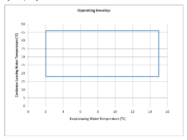
Other limits are: Maximum startup evaporator inlet fluid temperature, 32°C Maximum non-operating inlet fluid temperature, 38°C
