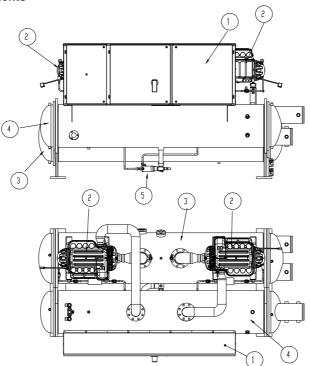
1. **Electrical panel**: Contains all electrical (main disconnect, inductances, filters, fuses) and electronic components.
